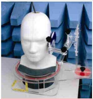
To the left is the science that determines wireless safety. Fluid is poured in the top where a temperature probe measures heat with EMF absorbed **by cell phone only**.
